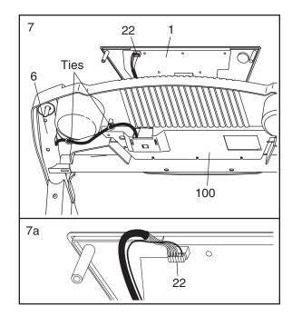
8. Set the Console (1) on the Console Base (100). Insert the excess Wire Harness (22) into the large hole in the side of the Right Handrail (6). Securely tighten the plastic ties on the bottom of the Console Base to prevent the Wire Harness from slipping. Then, cut off the ends of the plastic ties.
